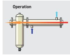
Compressed air or gas passes through the cooler tubes. Cooling water passes around the tubes in counterflow.
